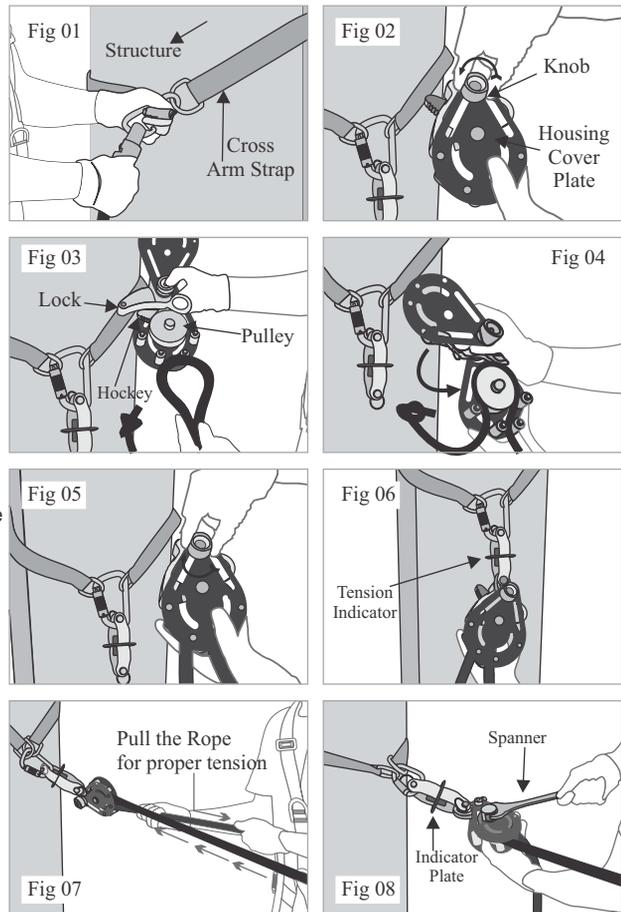
Step 6 : Use an open end spanner of 0.944 inches provided along with tensioner to give appropriate tension to the lifeline. Plate of Tension indicator will start to rotate freely once the required tension has been achieved in lifeline. Now, O rings/ pass through carriages can be used as mobile anchors for the workers. Fig. 08
